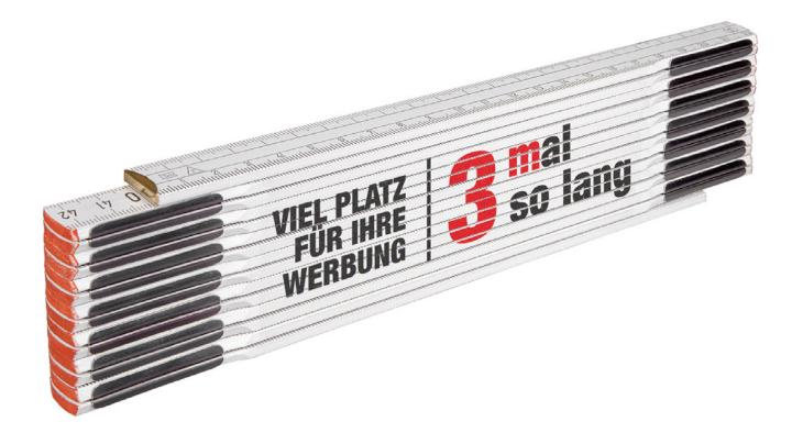
Wooden folding rule made of beech wood, 3 m, with integrated steel springs, concealed rivets and joints made out of Swedish steel. They have been heat treated and are epoxy painted. A compact side offers a perfect surface for your promotional imprint.
